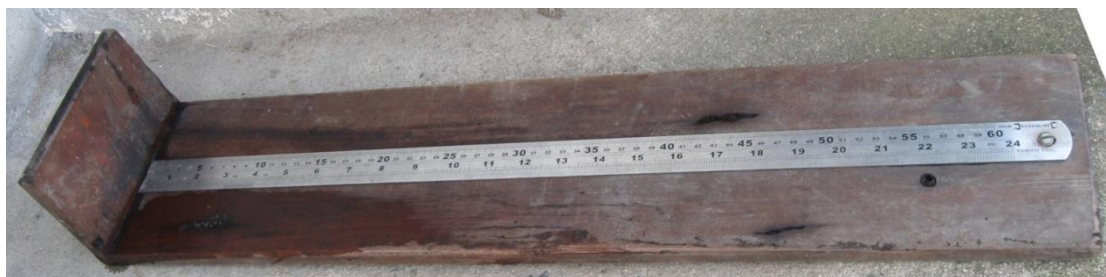
Figure 3.7. Locally-constructed fish measuring board.
