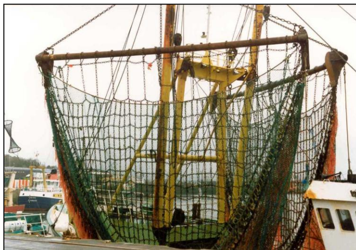
Figure 1.5 A beam trawl (Source: Jim Ellis).
